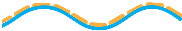
Side View: Small guard plates allow for a high degree of flexibility while providing tough protection
