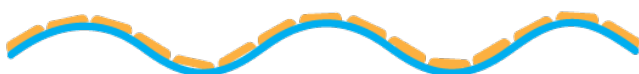
Side View: Small guard plates allow a high degree of flexibility while providing superior protection
